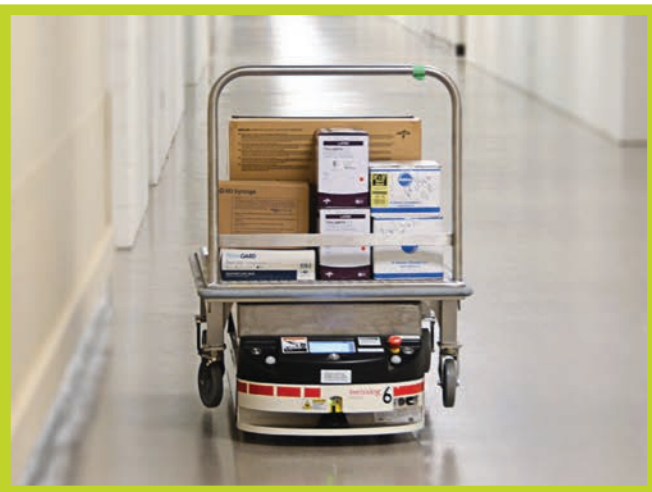
An automatic guided vehicle, or AGV, delivers supplies within the hospital.
